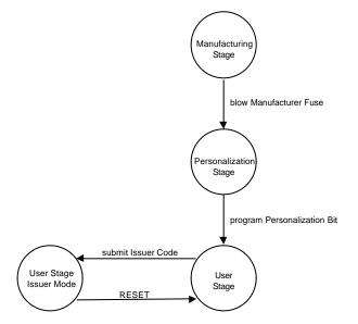
The actual chip life cycle stage is determined by the card operating system immediately after a reset. The life cycle stage does not change during the operation of the card.
